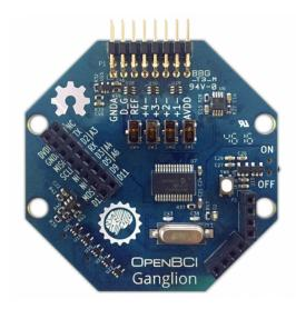
Figure 2.4: ECG monitor: OpenBCI Ganglion Biosensing Board.
