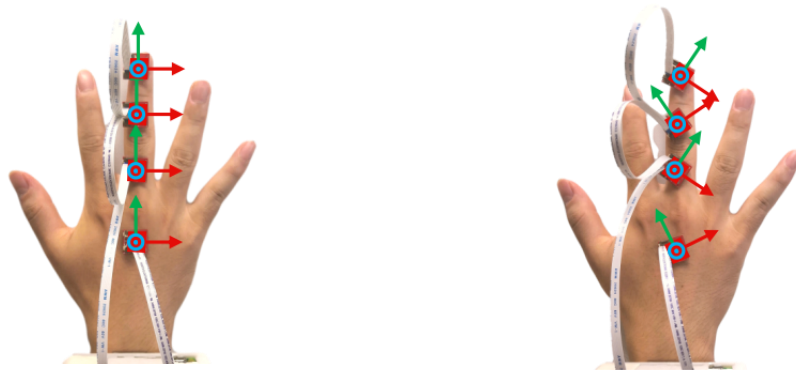
Figure 3.15: Two types of mounting orientations include alignment (0 degrees offset) and misalignment (about 30 degrees offset).
