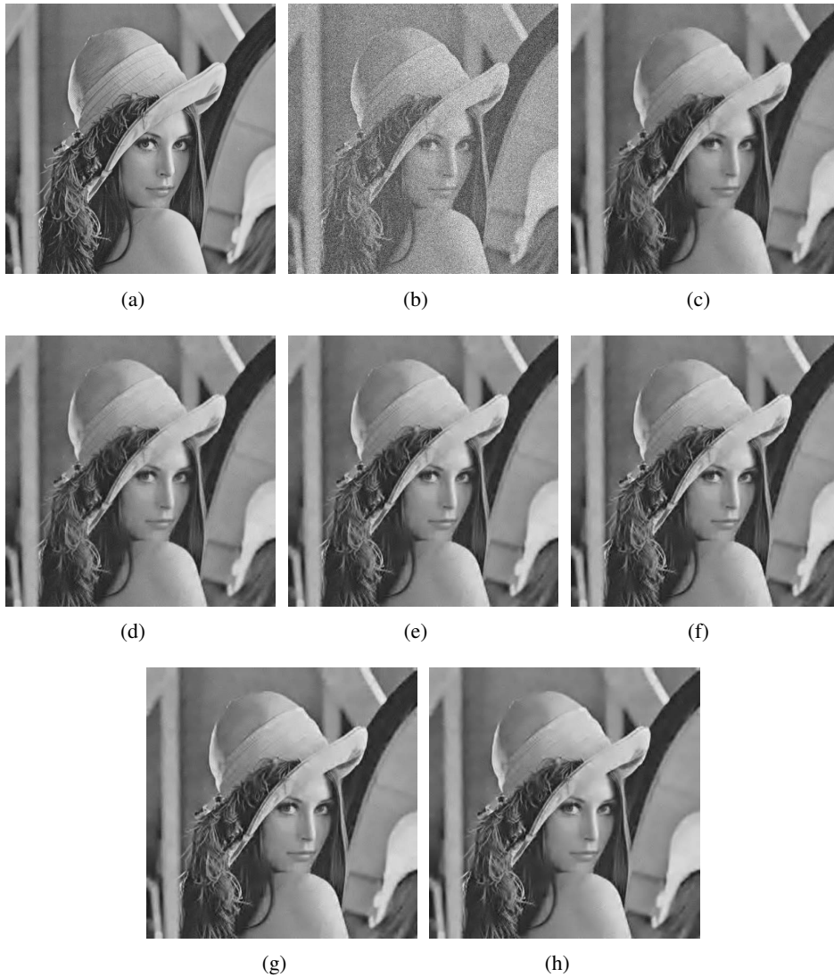
Figure 4.8: Image-denoising result: (a) Original image; (b) Noised: 20.17 dB; (c) ISTA: 29.13 dB; (d) WISTA0.9: 29.88 dB; (e) WISTA0.7: 30.79 dB; (f) WISTA0.5: 31.01 dB; (g) IHTA: 31.00 dB; and (h) OMP: 30.93 dB (from top left to bottom right)
