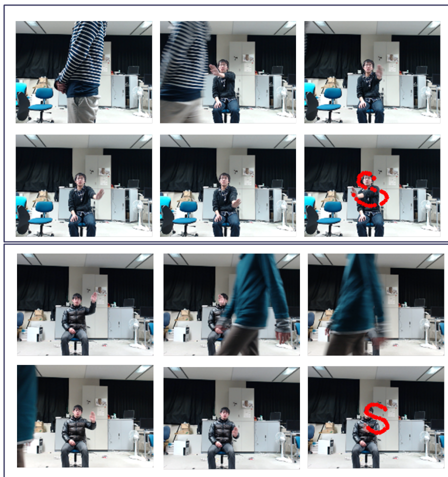
Figure 8 The upper figure shows occlusion occurring at the beginning of drawing the ‘S’ character. The lower figure shows occlusion occurring during the middle period. TSCDP recognizes character gestures correctly in both cases.
